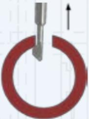
Moving back with feed F100. Thereby the burrs are removed.
