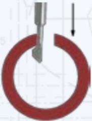
Moving in the hole with feed F500 until the sharp slope of the blade is through.
